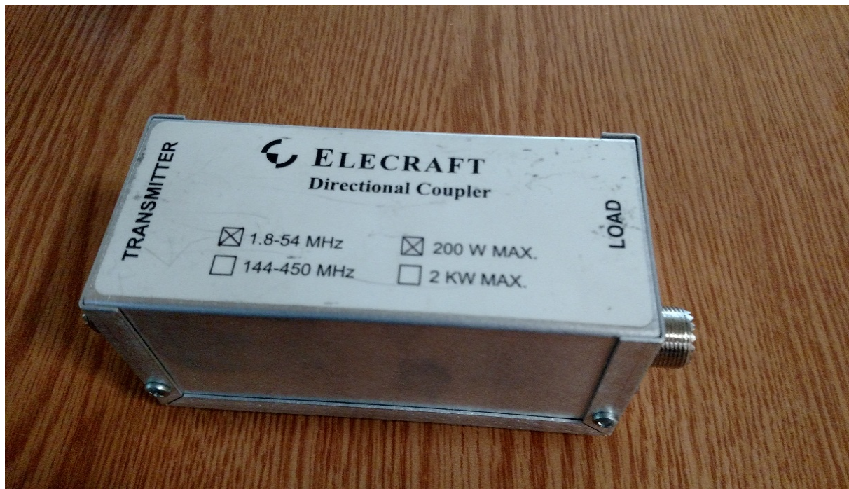
Elecraft DCHF-200 Directional Coupler Used For Auto-Tune Feature
